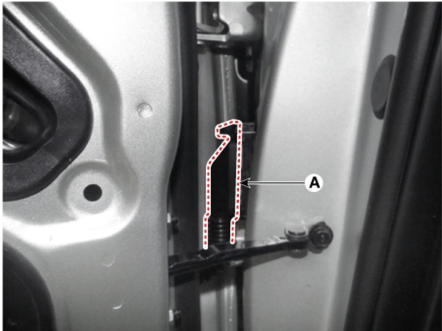
10. Loosen the front door latch mounting screws (A).
